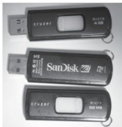
Figure 9-8 USB drives that implement the U3 standard
