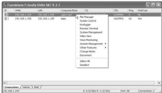
Figure 6-2 Gh0st RAT Command & Control screen
