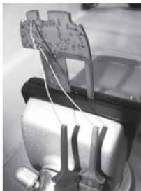
Figure 9-18 A PCB with attached wire acting as test points for logic analyzer
