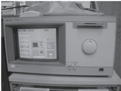
Figure 9-15 A logic analyzer views signals traversing a bus.
