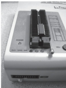
Figure 9-20 A B&K Precision 866B EEPROM programmer with microcontroller inserted for programming
