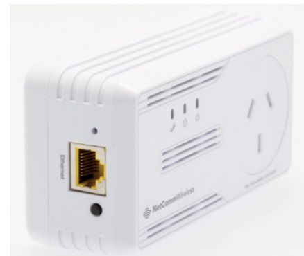
In lieu of running Ethernet cables all over the place, powerline solutions like the Netcomm Wireless NP507 can provide a neat way to link your second router back to your first.
