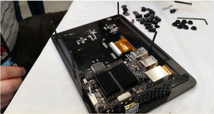
Figure 6 - Insert the remaining 4 screws into the tablet cover, and place 3 spacers over top of the screws running through the ODRROID-C
