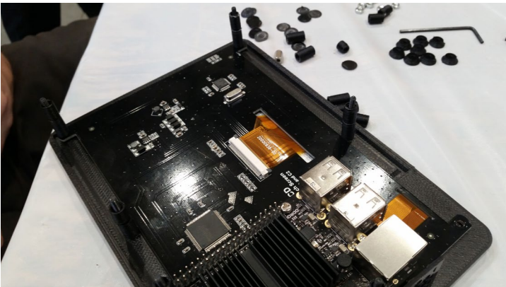
Figure 7 - Place a pair of spacers over top of the 4 tablet cover screws, which may need to be trimmed slightly with a utility knife in order to ensure the best fit
