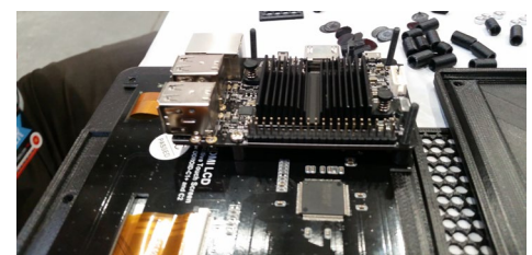
Figure 4 - Place the ODROID over the screws, on top of the spacers, so that the board's top is facing away from the screen
