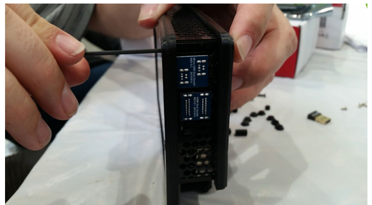
Figure 11 - Tighten the screws using the included hex wrench, making sure not to overtighten them
