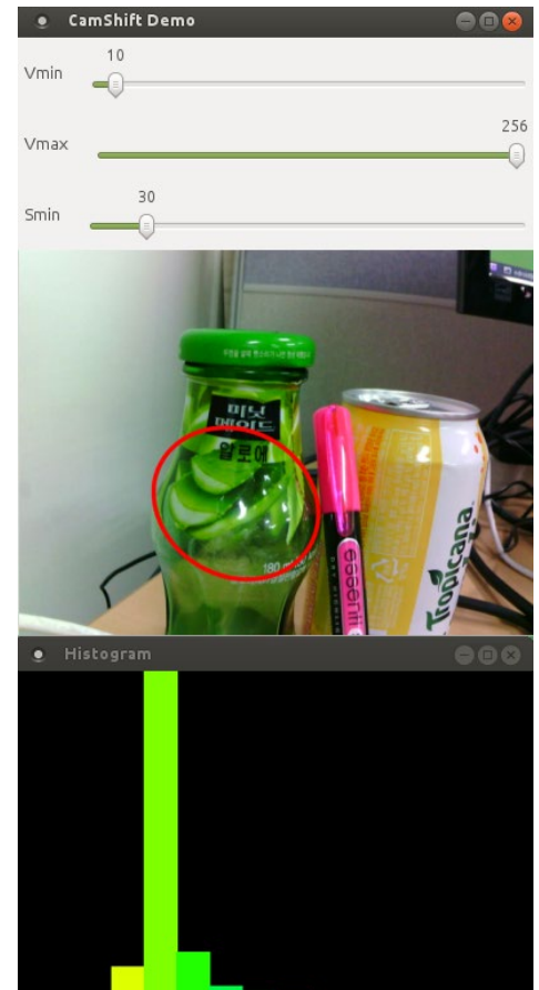
Figure 5 - The target area being tracked and the histogram of color components
