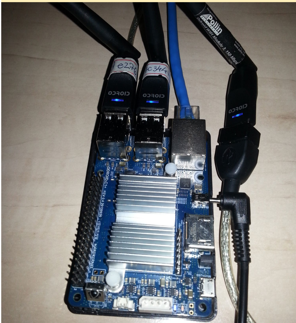
Figure 6 - Wifi Module 3 is thicker than the USB port and requires a cable to be attached
