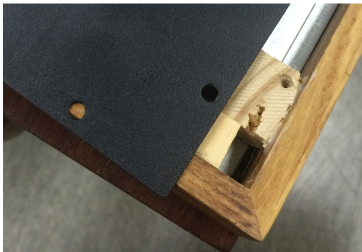
Assemble the steel plate to the bezel frame with screws
