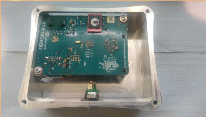
Figure 6 - ODRROID-XU4 inside the top cooling area
