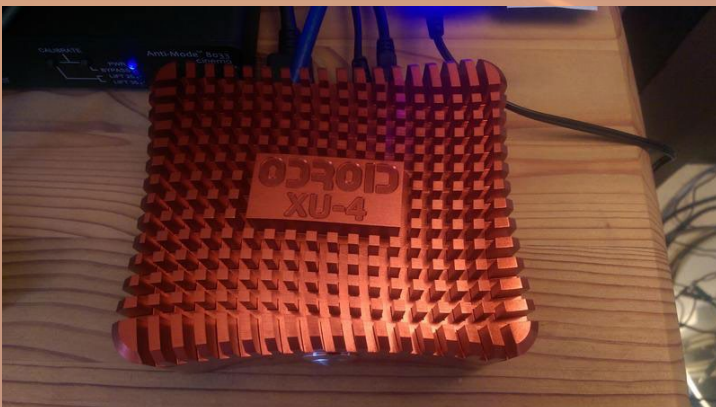
Figure 8 - The final product was done with red anodizing
