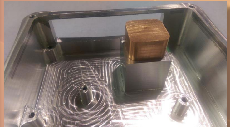
Figure 4 - The copper core attached to the inside of the case for passive cooling
