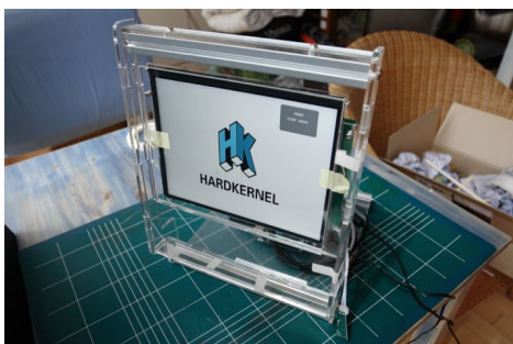
Figure 5 - LCD panel mounted inside front of case
