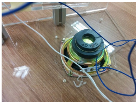
Figure 7 - Internal speaker mounted on front of case
