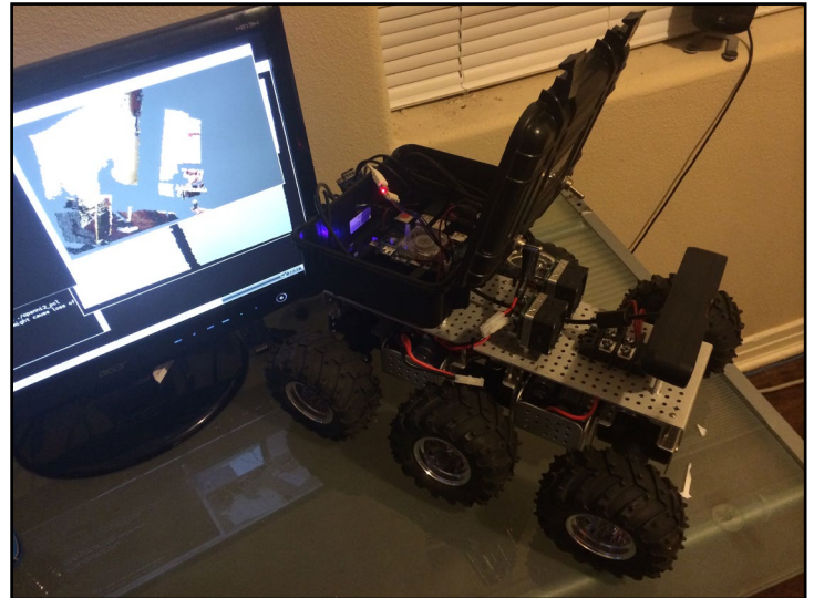
This robot runs on an ODROID-XU, is made from readily available parts, and loves rough terrain.
