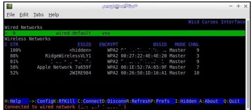
WICD allows the ODROID to easily connect to any wired or wireless network
