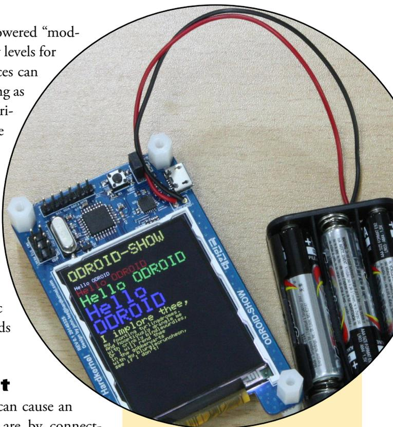
The ODROID-SHOW LCD Panel with optional battery pack
