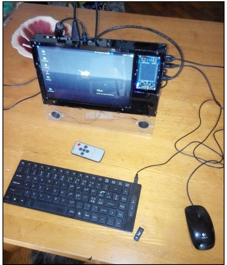
The finished laptop case, with speakers installed at the bottom of the clear plexiglass front, a handy I/O shield for quick hardware prototyping, and a beautiful 10.1" HD monitor
