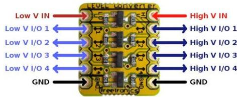
**Freertronics Logic Level Converter Module with 4 IO Ports**
