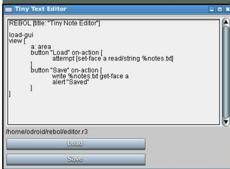
As you can see, Rebol's code structure is pretty free-form. The Tiny Text Editor is laid out differently than the Tiny Note Editor, but mostly because the buttons' on-action blocks are split into lines based on the actions being specified.
